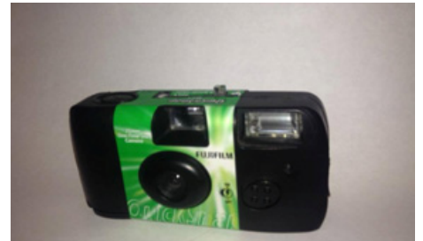
Front view showing lens, view finder and flash.
