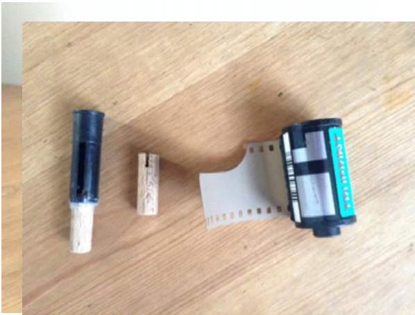
Photographic film and one of the wooden winders combined with a plastic kit camera winder.
